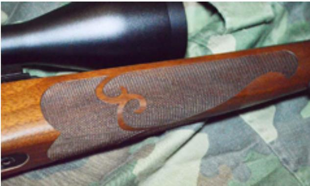
*“Checkering” the wood of a gunstock provides extra grip.*
